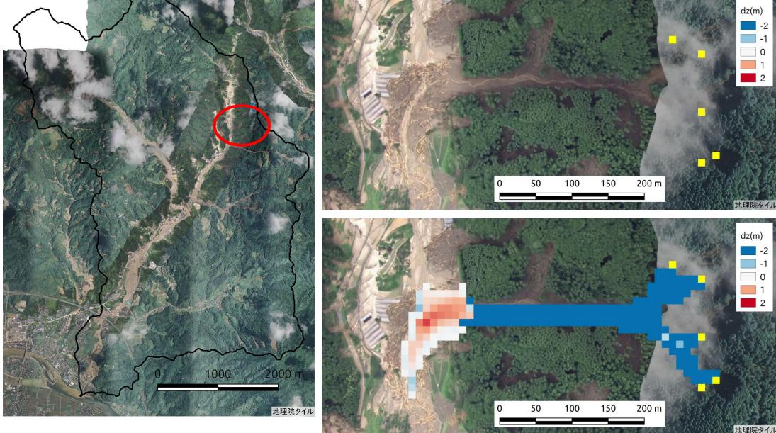
Spatial distribution for erosion and deposition resulted from debris flow
