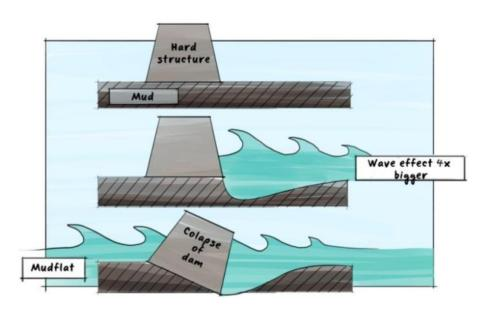
Waves reflect on hard structures, increasing eroding force
